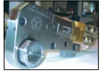
Low cost step-down sleeves are available in all sizes.
